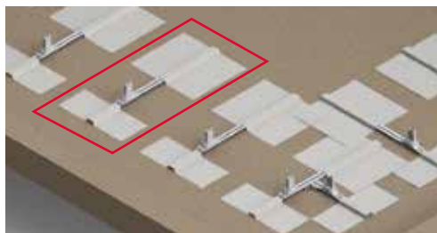
Step 2: Install load-bearing plates and railing feet
